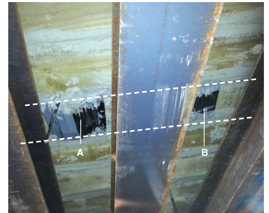
Figure 3. Deployed SmartPlank at TCR Stair 14. (A = wireless node, B= strain gauge and temperature sensor)
