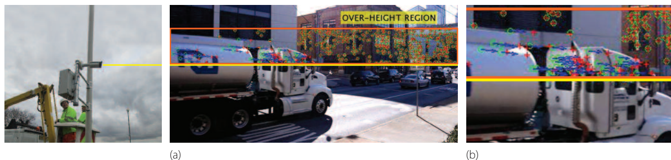
Images show: (a) Camera system installed at Fairlop Station in London. The camera is installed at the same height as the bridge clearance; when calibrated, the camera behaves like a laser-beam and detects moving objects above the over-height plane; the over-height plane (3D), i.e., line in camera view (2D) and region of interest (ROI) are annotated in yellow and red, respectively; the ROI is optimally positioned above the over-height plane to minimise the amount of processing required; (b) zoomed in view – the moving over-height features are detected and tracked using Kanade–Lucas–Tomasi algorithm.
