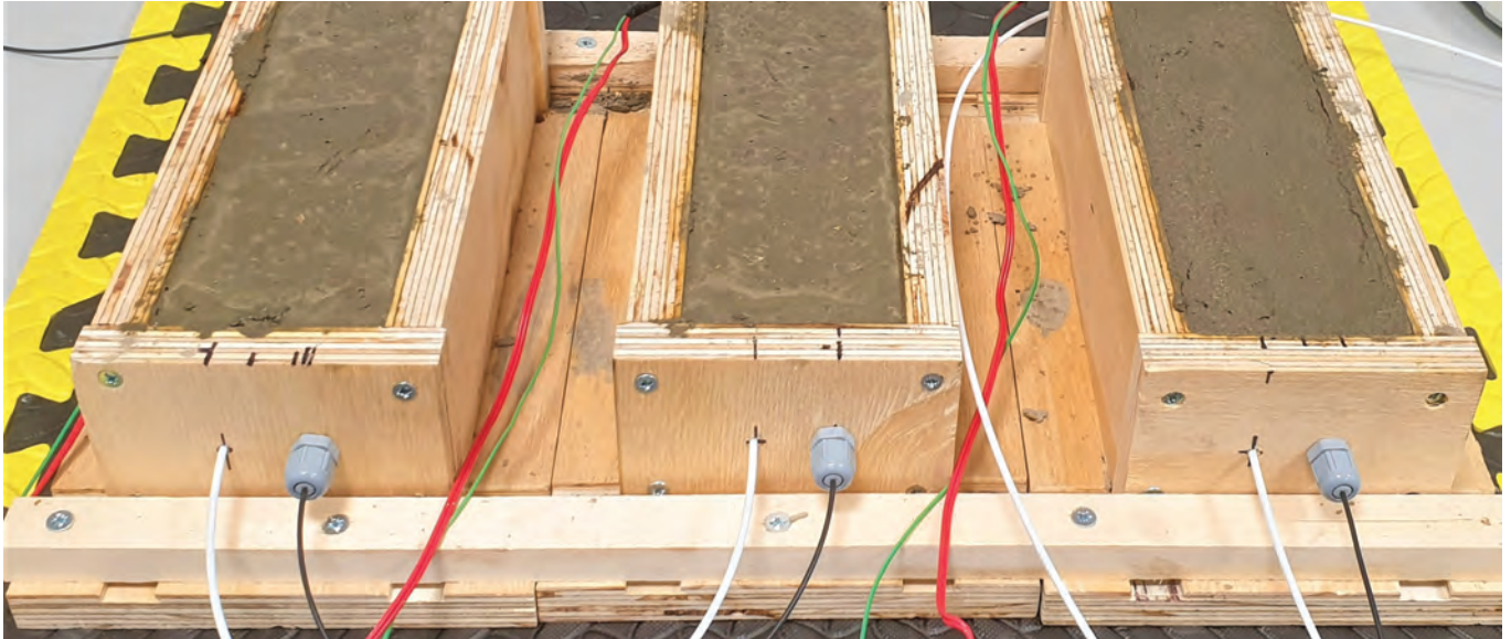
Concrete samples with embedded fibre optic sensors to measure strain and temperature
