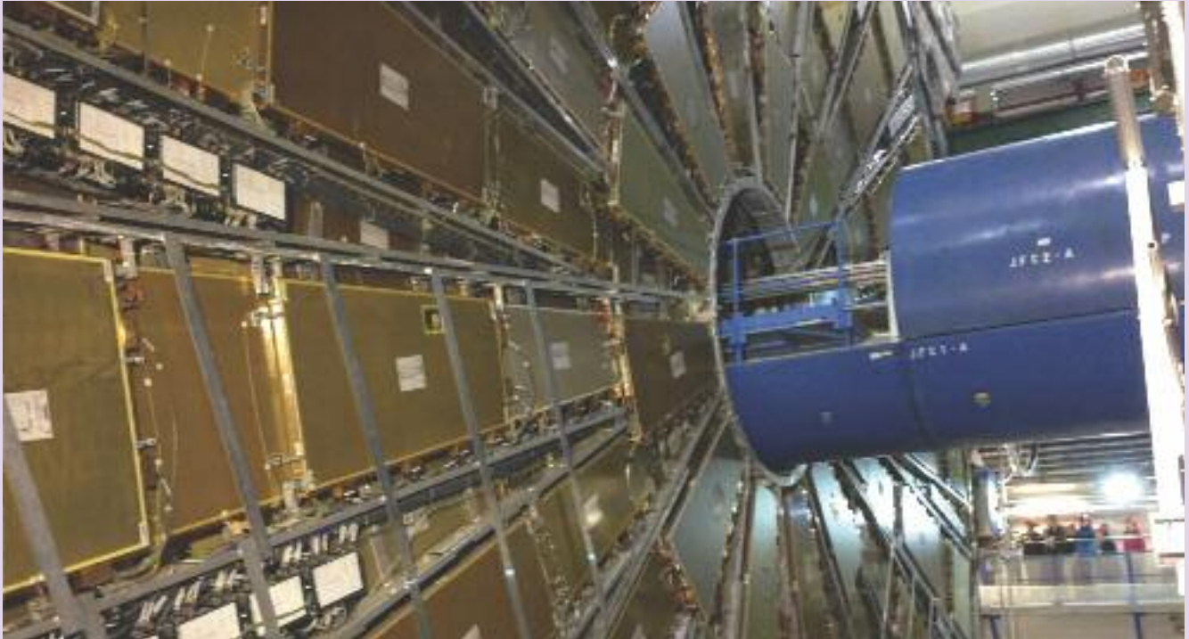
The ATLAS detector, one of the particle detector experiments constructed at the Large Hadron Collider (LHC), CERN
