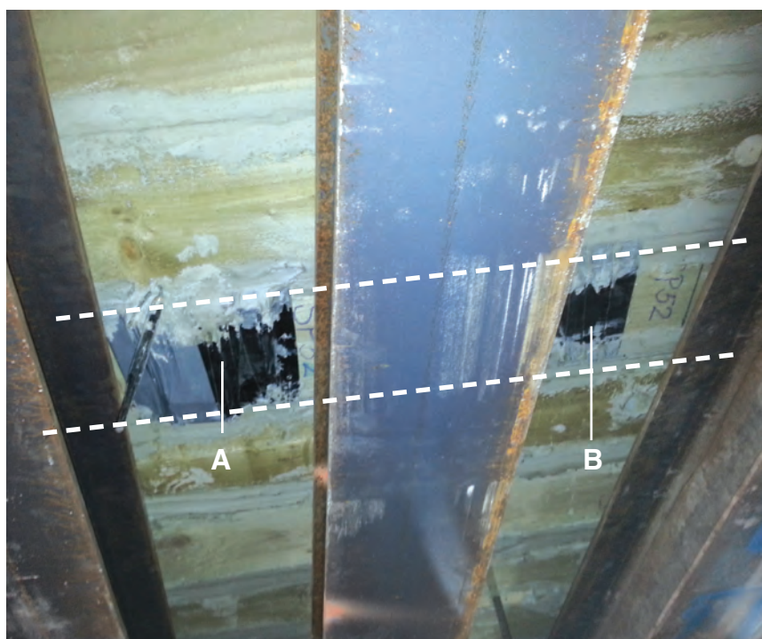
Figure 3. Deployed SmartPlank at TCR Stair 14. (A = wireless node, B= strain gauge and temperature sensor)
