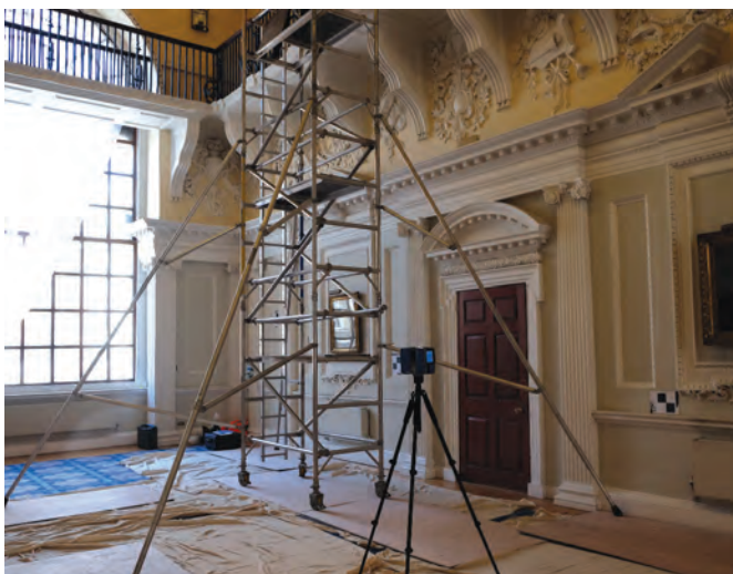
Laser scanning at Mansion House
