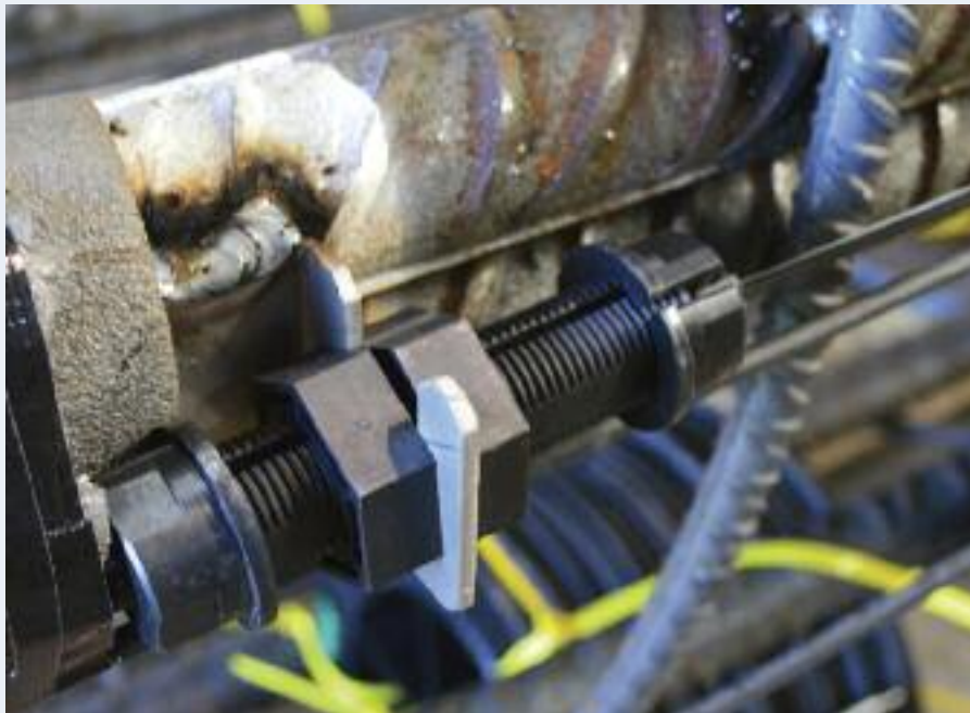
A pre-tensioning clamp and fibre optic cable on a reinforcement cage
