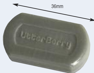
Ultra low power 'UtterBerry' wireless sensor mote
