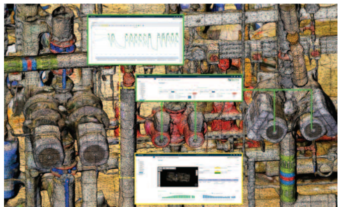
Figure 2: View of the BIM Model of IfM Plant Room with information about components displayed
