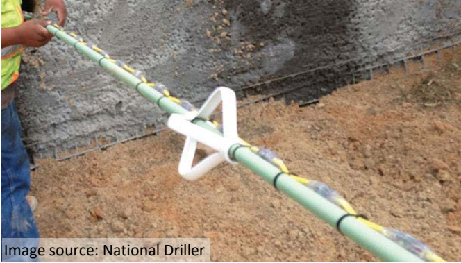
Thermal Integrity Profiling thermistor array
